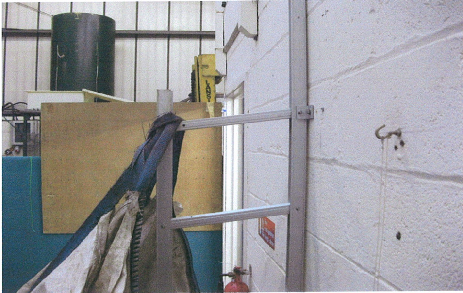
Final vertical test with 345kg. Rung angle 7.5degrees
